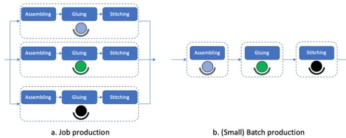
Figure 2. Changing in production method and layout
